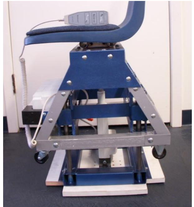
Fig. 13.4. Chair in lifting mode.
