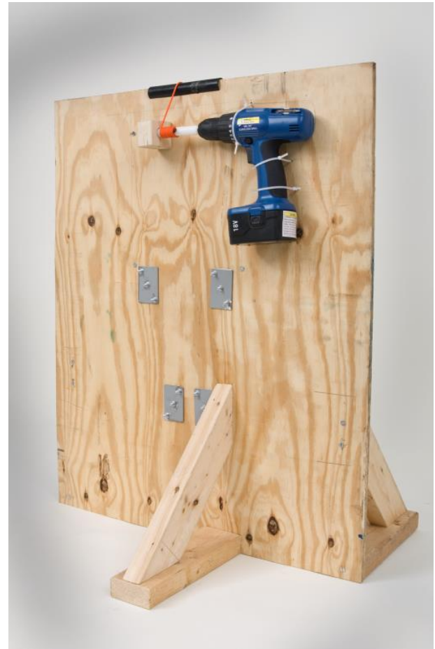
Fig. 11.50. Motor to Move Cabinet.
