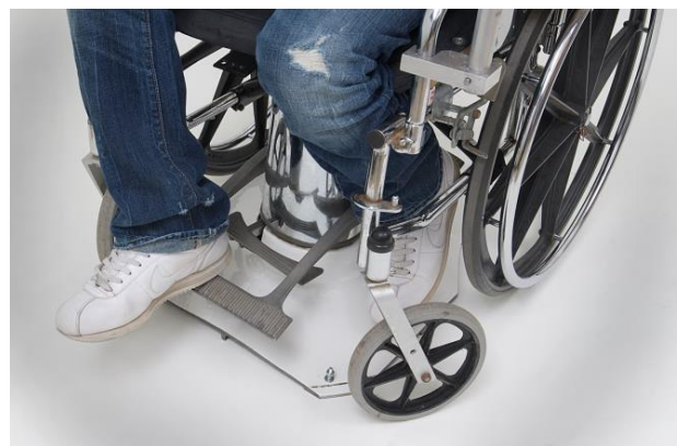
Fig. 11.30. Close up of Pneumatic Lift System.
