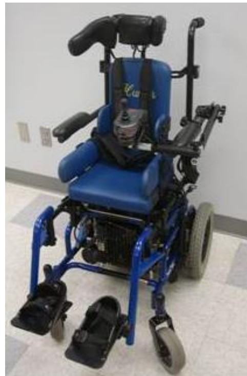
Fig. 14.5. Photo (left) of the adjust-able joystick mount, which was designed to be attachable at two sites permitting hand control (right) or foot control.
