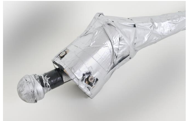
Fig. 11.87. Leading Tip of Smart Cane with Sensors.
