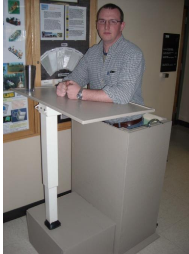
Fig. 14.8. Example adjustable height standing boxes completed by the freshman engineers in EGR 100 Introduction to Engineering. Each of these devices, along with one other (not shown) were selected for use by staff at LINCPoint to serve adults with cerebral palsy.
