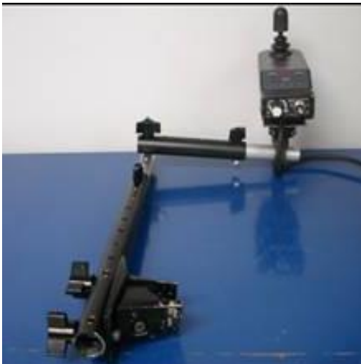
Fig. 14.5. Photo (left) of the adjust-able joystick mount, which was designed to be attachable at two sites permitting hand control (right) or foot control.
