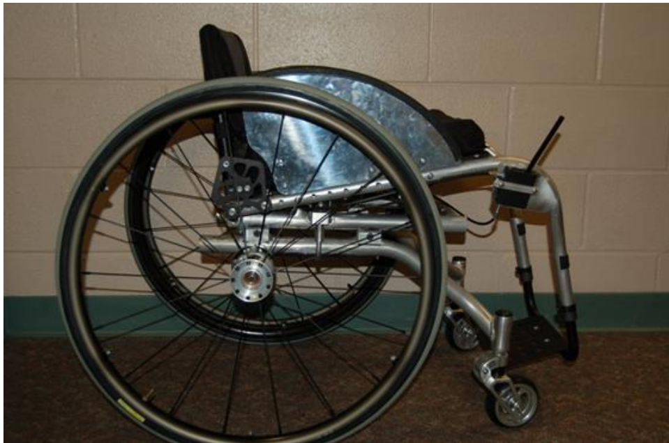
Fig. 20.3. The completed prototype in the hill climbing position.
