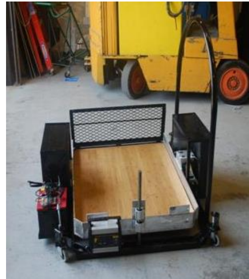
Fig. 14.1. CAD drawing (left) and completed prototype wheelchair lift (right) for LINCPoint. The design features battery powered car jacks for lift, reduced weight as compared to an earlier design, and spring loaded casters for mobility when not in use.
