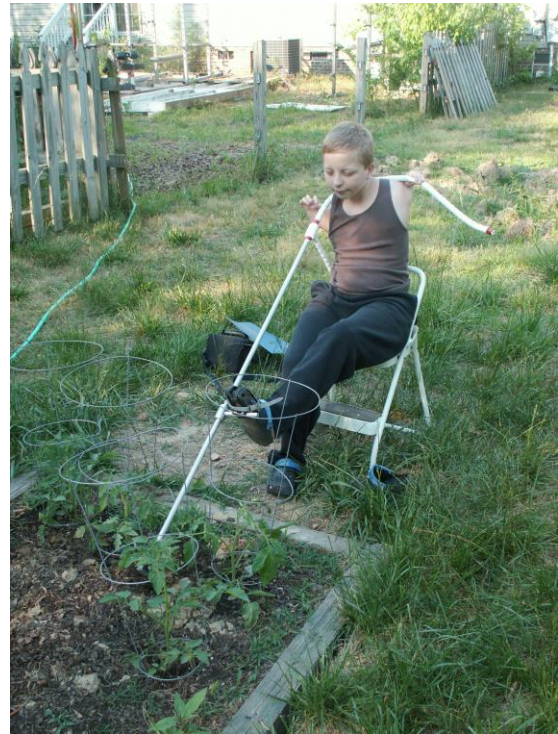
Fig. 7.25. The client using the integrated body-rod tool for hoeing.
