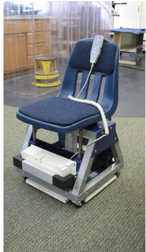
Fig. 13.1. Whisperlift chair with control cable.
