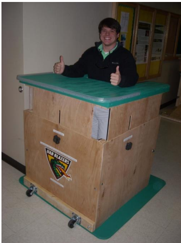
Fig. 14.8. Example adjustable height standing boxes completed by the freshman engineers in EGR 100 Introduction to Engineering. Each of these devices, along with one other (not shown) were selected for use by staff at LINCPoint to serve adults with cerebral palsy.
